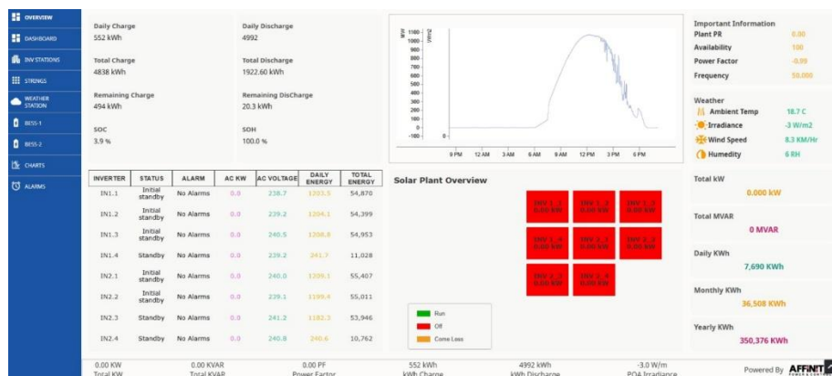
Figure 14: PV SCADA User Interface.
