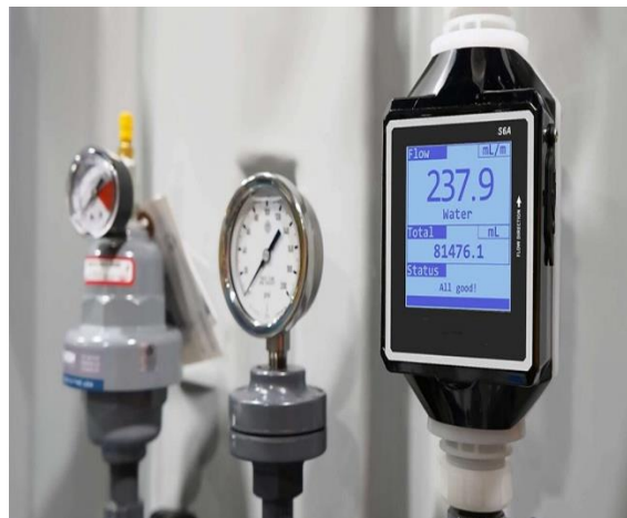
Figure 26: Water flow meters.
